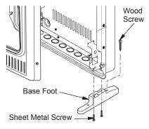
Figure 13 - Installing Base Feet
